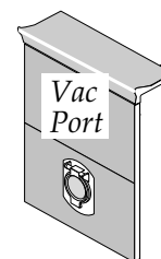
Figure 15: Typical Dedicated Vacuum Port.
